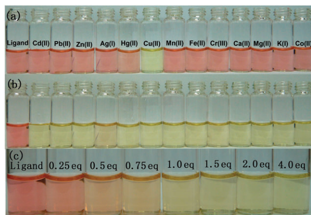
Fig. 1 (a) The color change of 1 (12.5 \mu M) upon adding 1 equiv. of various metal ions. (b) The color change of 1 (12.5 \mu M) upon adding 1 equiv. of copper ions in the presence of various other metal ions. (c) The color change of 1 (12.5 \mu M) upon adding various amounts of copper ions to the aqueous buffer.
